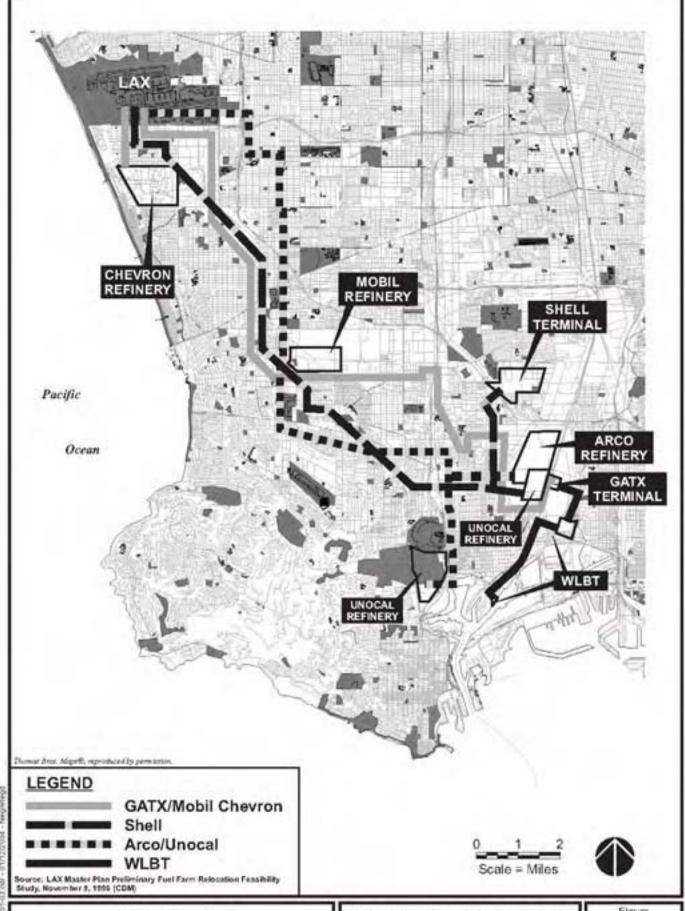
LAX Master Plan Final EIS/EIR Oil Refineries, Terminals and Pipelines Serving LAX Figure F4.17.1-3
