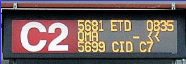
Ramp Information Display System (RIDS) have been incorporated into the Bradley West design at each of the new gates. Each RIDS shall be mounted on the exterior wall of the concourse to help ground crews, pilots, flight attendants and ramp agents ensure ground traffic flows efficiently. RIDS uses can include flight numbers, aircraft tail numbers, estimated time until departure/arrival and design-
