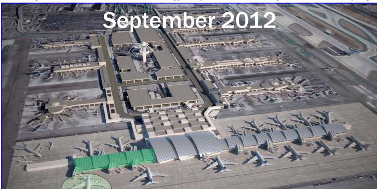
The next step following the 12/12/12 opening will be the demolition of the existing south concourse to allow completion of the Demolition of the morth concourse, clearing the way for the final construction east apron for the new south concourse. The south concourse east gates are anticipated to become operational in August of 2013.
