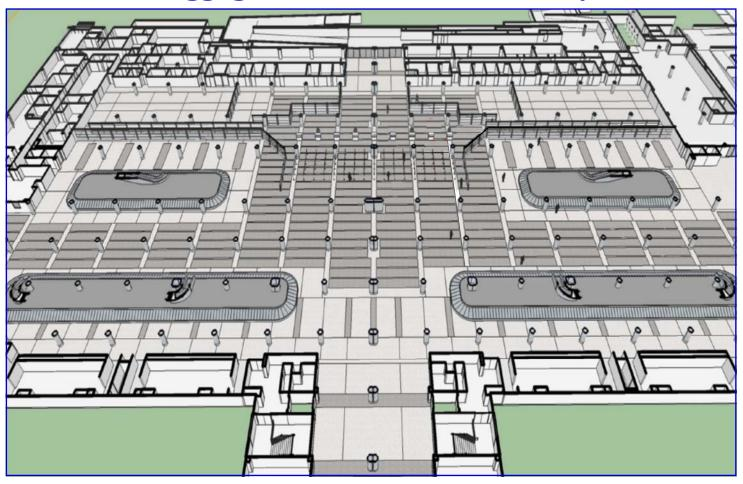
In addition to the SSCP construction and impacts to the departing passenger, the TBIT Renovation includes renovations to the old baggage claim and CBP facility. This Level 1 renovation will include the removal of all CBP primary booths, reconfigu-
