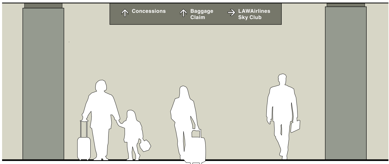
Figure 31: Directions to tenant passenger lounges may appear on airport directional signs by request to LAWA.
