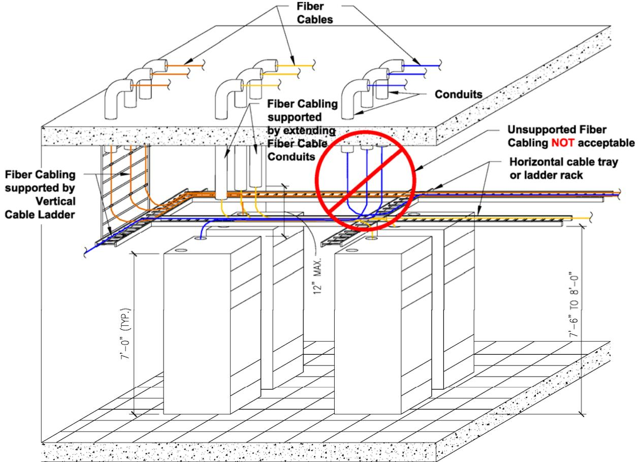
**Vertical cable tray supports cables to the horizontal cable tray when conduits do not reach.**
