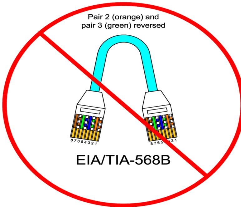
**CAT 6/6A cable shall follow the EIA/TIA-568A wiring standard.**
