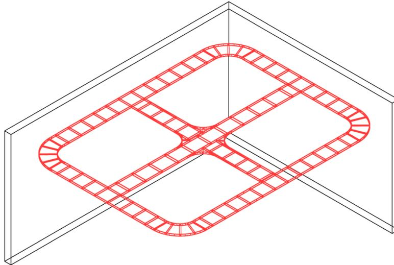
**Cabletray/Ladder Rack is required around the perimeter, over the cabinets, and across the room.**
