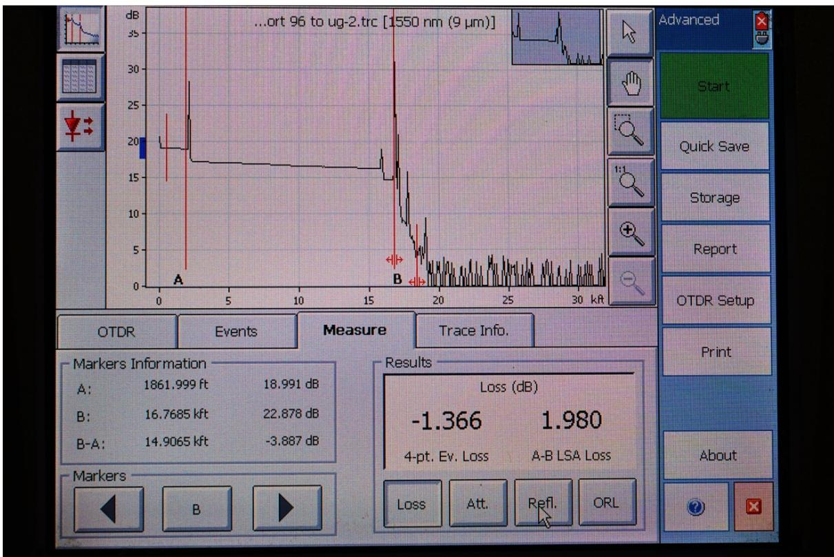
Picture of a typical OTDR tracing.
