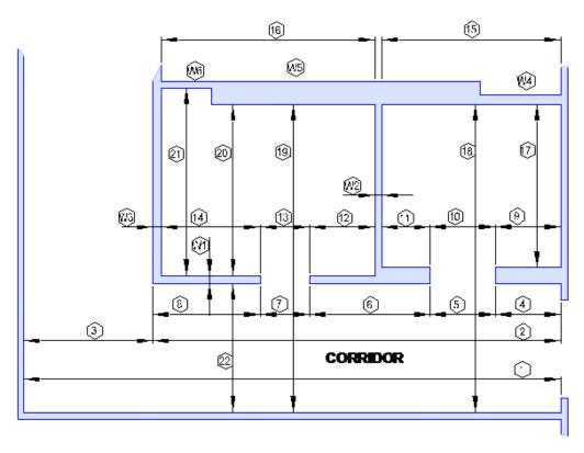
Figure 9. Wall thickness measurement guidelines
