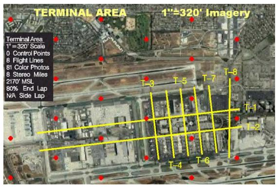
Figure 3. Terminal Area Flight line locations
