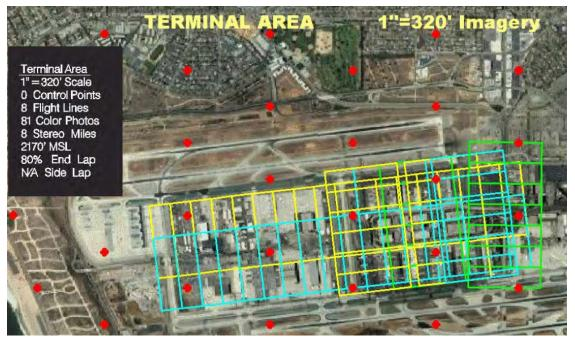
Figure 2. Terminal Area Model Limits
