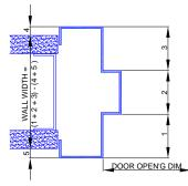
Figure 13. Door jamb - typical measure points
