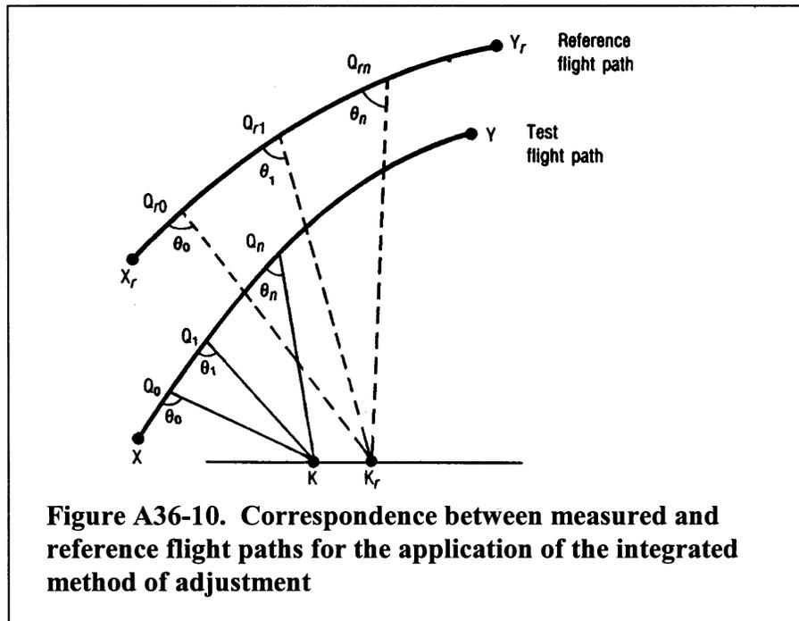
(1) XY represents the portion of the measured flight path that includes the noise time history relevant to the calculation of flyover and approach EPNL;  $X_rY_r$  represents the corresponding reference flight path.
