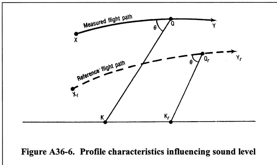
and reference noise propagation paths, Q<sub>r</sub> being determined from the assumption that QK and Q<sub>r</sub>K<sub>r</sub> form the same angle  $\theta$  with their respective flight paths.
