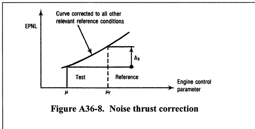
**Figure A36-8. Noise thrust correction**
