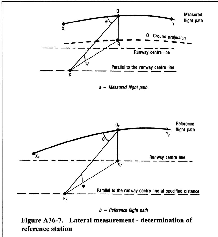
**Figure A36-7. Lateral measurement - determination of reference station**
